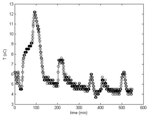
Fig 1 Temperature variation in a domestic refrigerator
