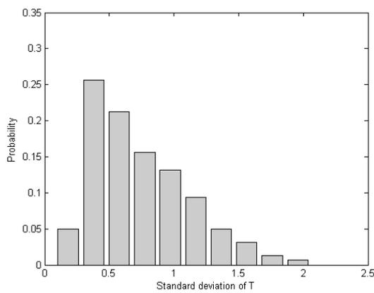
Fig 3 Probability Distribution of standard deviation in temperature profiles in domestic refrigerators
