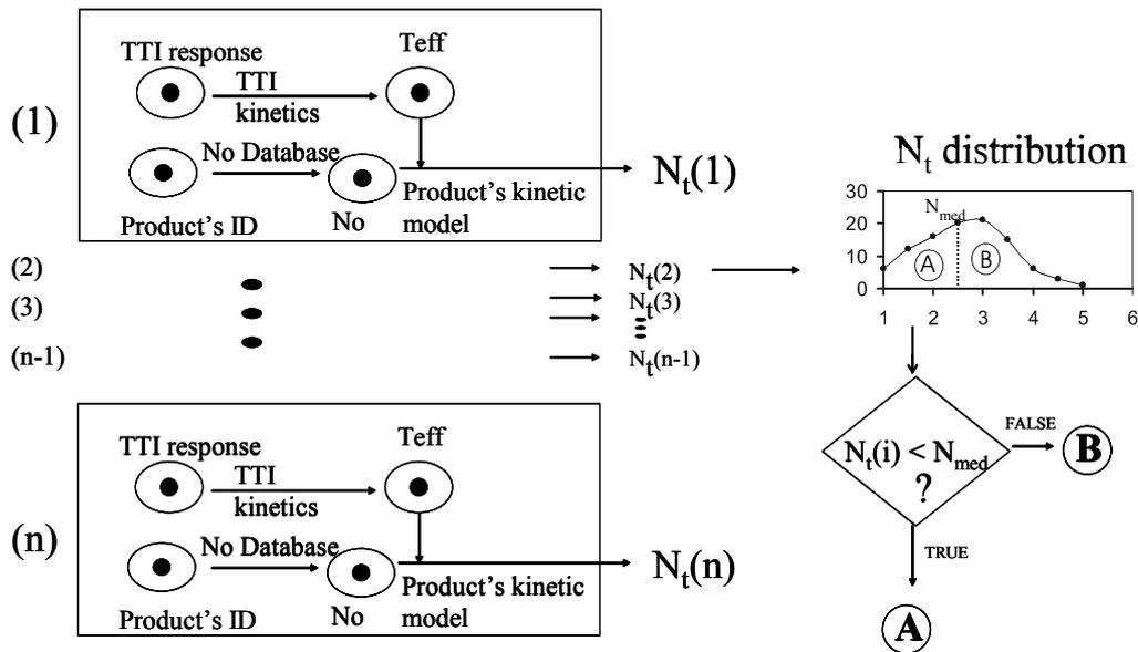
**Fig 1** SMAS logical diagram of the decision making routine at important points of the distribution chain. The extent of pathogen growth  $N_t$  is calculated for all meat units and the decision for further handling is based on the position of each unit within the distribution, compared to the median growth ( $N_{med}$ )
